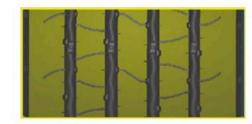
Straight groove and 5-rib design help to even wear and reduce rolling resistance.
